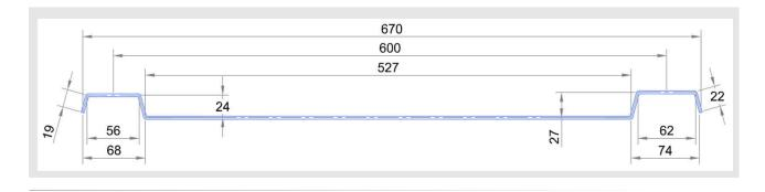
Our Modular Roof System is a high quality, extruded, plastic sheet made of polycarbonate (PC). This is suitable for a range of external roofing applications combining a smooth easy to clean surface, good fire performance and chemical resistance. Sheets should be continuously supported on rafters at 5 degrees(min) and secured with specified fasteners at 500mm ctrs. Sheets must be pre-drilled with 12mm dia holes to allow thermal movement.
